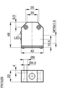
Inductive Sensors BES 516-346-H2-Y 22 x 42 x 48 normally-open Sn=5mm shielded
